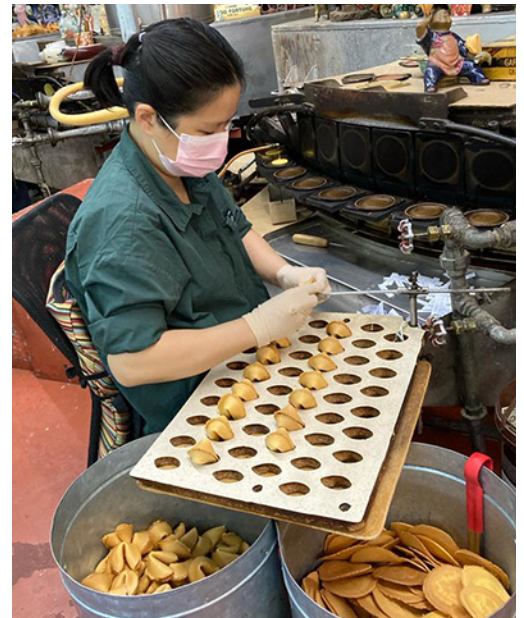
A worker at the company makes fortune cookies by hand and bakes them on an antique, cast-iron rotating griddle.
